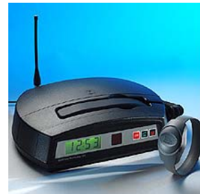
GSM Site Monitoring Unit (GSMU)
